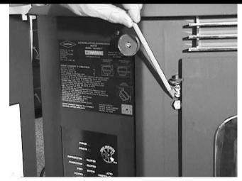
Fig. 15: Draft Meter bolt hole location
